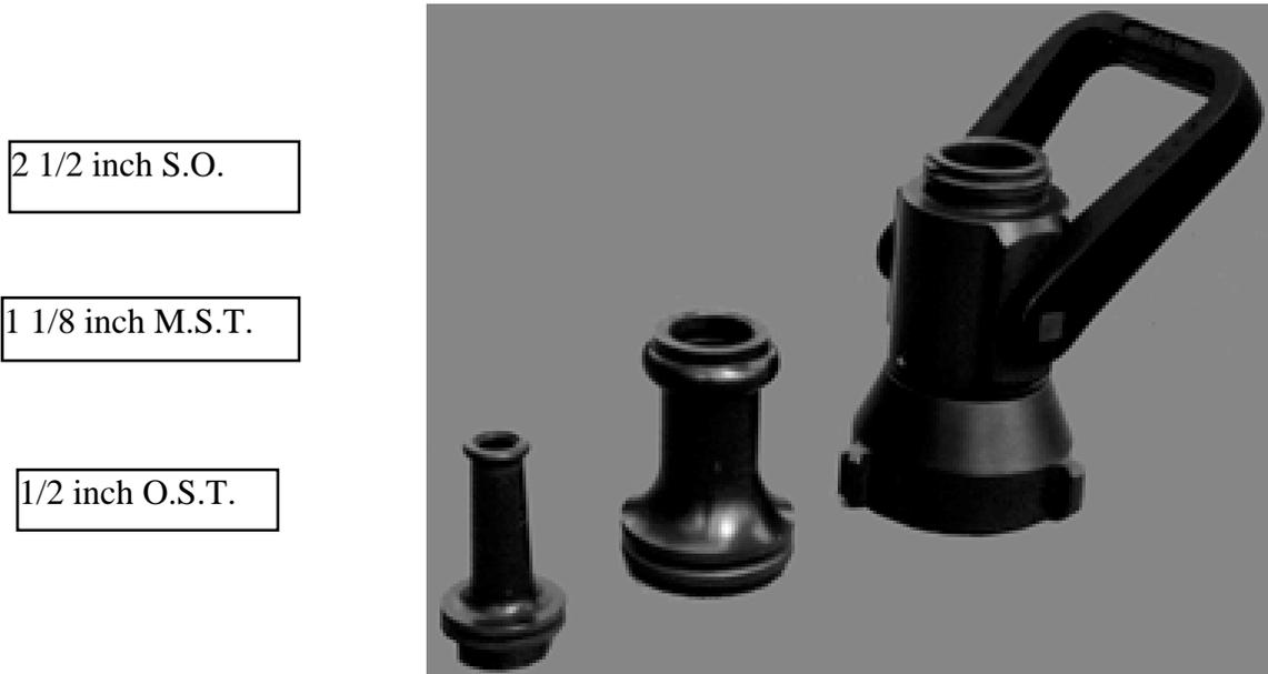
**Fig. 2-2** - 2 1/2 inch solid stream nozzle with 1/2 inch outer stream tip and 1 1/8 inch main stream tip for use on 2 1/2 inch handline.
