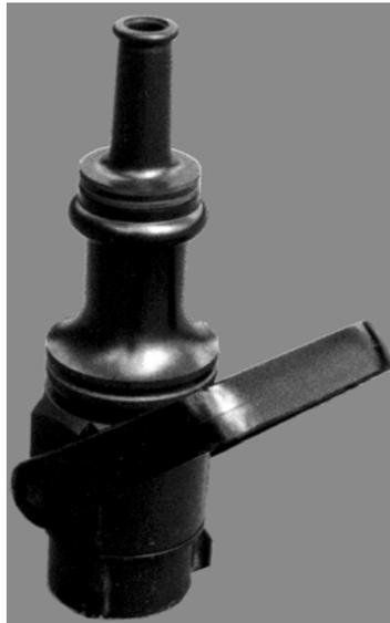
**Fig. 2-1** - 1 1/2 inch solid stream nozzle with 1/2 inch outer stream tip and 15/16 inch main stream tip for use on 1 3/4 inch handline.
